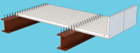
Typical EMJ Permadec Diaphragm panel installed on concrete beams
