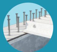
This sealant has been specially designed to stop ingress of water during the life of the structure and also to prevent any grout loss when pouring. It has being tested to prove excellent adhesion against two substrates, the maximum force required to remove the panel after sealing is equivalent to 6.15kN/m run of panels.
